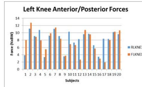
Figure 2. Forces shown are the average of the peak forces observed in five steps and demonstrates forces observed in the left knee. Positive values for (a) designate forces in the lateral direction and negative values for (a) designate forces in the medial direction. Positive values for (b) designate forces in the medial direction and negative values for (b) designate forces in the lateral direction.
