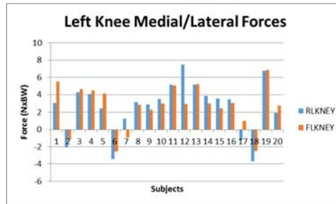
Figure 1. Forces shown are the average of the peak forces observed in five steps and demonstrates forces observed in the left knee. Positive values designate forces in the anterior direction and negative values designate forces in the posterior direction.
