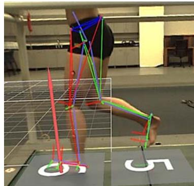
Figure 3. Rearfoot strike video capture with 3-D overlay as viewed in the Vicon Nexus program.
