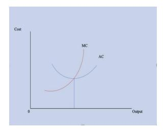
The production's minimum average cost corresponds to an optimal quantity produced x, for which the average cost equals the marginal cost. The marginal cost is secant with the average cost for the level of output such that production is done at the minimum unit cost:
