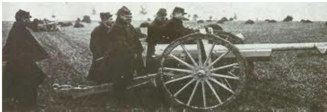
Figure 9: French Canon de 75 Modele 1897. (Notice the recoil tube under the gun barrel/this allowed the French gun to stay in place after each shot.
