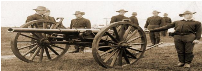
Figure 10: American M1897 3.2-inch gun. (No recoil system, after each shot the gun would roll back and the crew members would have to roll it back into battery and resight after each firing.
