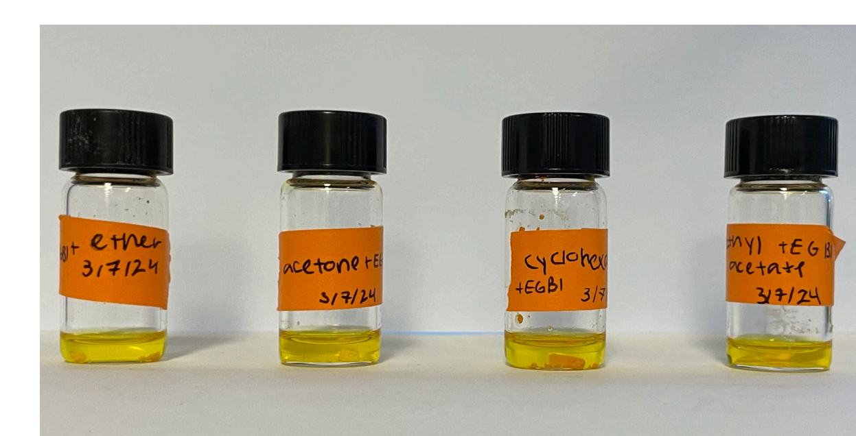
Figure 8. EGB1 in various solvents. From left to right: diethyl ether, acetone, cyclohexane, and ethyl acetate.
