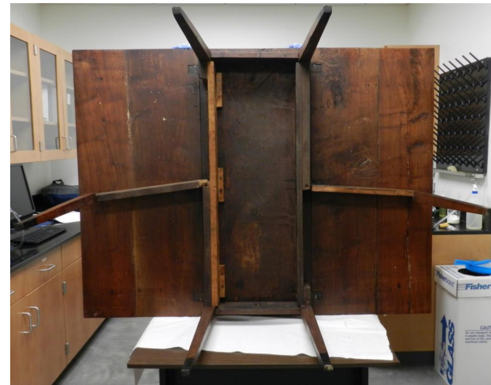
Figure 2. Surgical Table Expanded Bottom View View of the surgical table from the bottom, where a majority of blood stains were located. The table has two panels on the side that expand and legs that drop down to support it.
