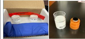
Figure 2. Company A SEM GSR Kit and Carbon Pad (Heinz & Morgan, 2023)
