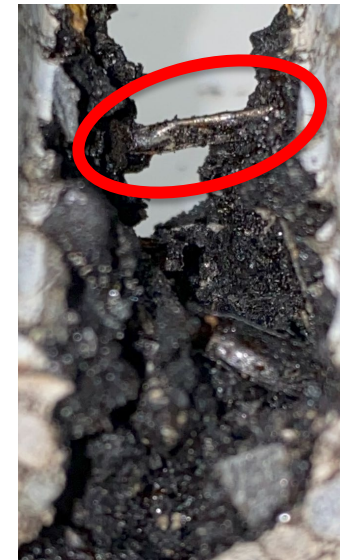
Figure 11 – Pulled out fibers at high temperature
