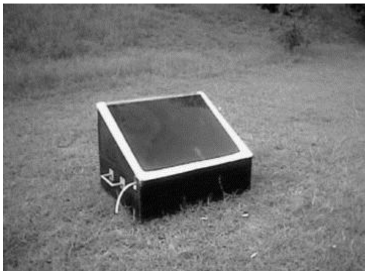
Figure 7 - Solar still being tested outside (Samee, Mirza, Majeed, & Ahmad, 2007)
