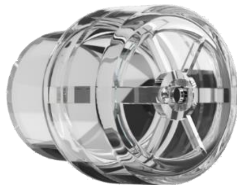
Fig. 1. CAD model of Original Passy Muir Speaking Valve (PMV) Design
