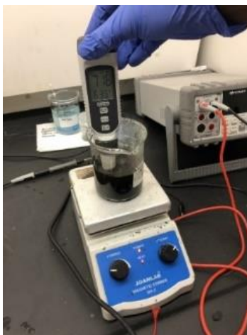
Fig. 3. Electroless deposition with increasing temperature.
