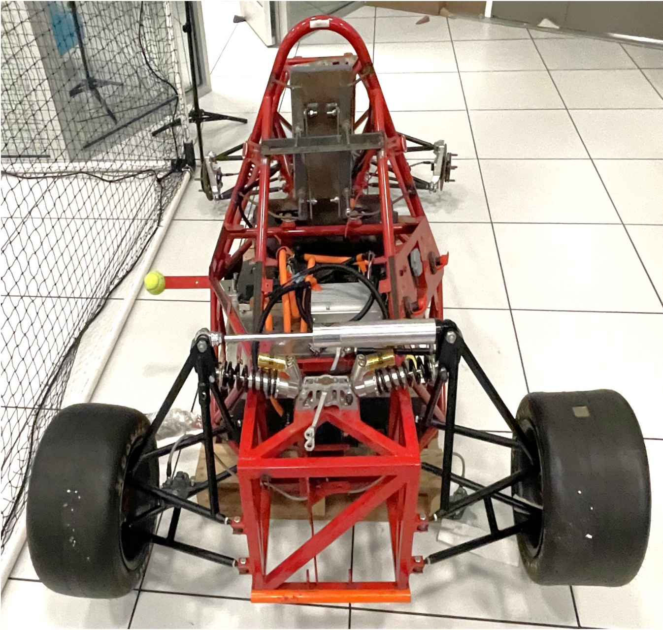
Figure 1. Electrical Vehicle with Third-damper Suspension The testbed is being designed and built for the system, which determines various aspects of the testbed's design, such as the width of the conveyor and the distance between the two conveyors. The car being tested has an estimated weight of 408.2 kg (900 lbs). (Photography by Kayden Bingham)
