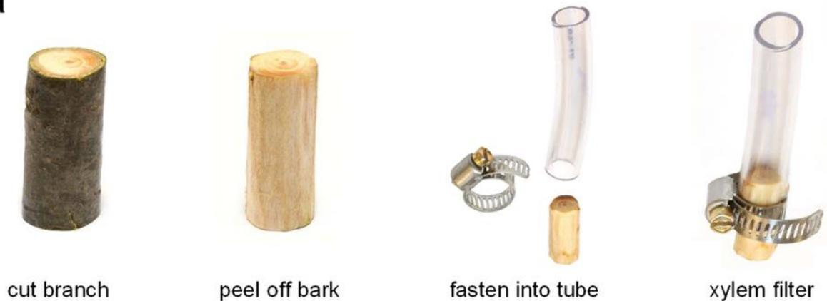
*Figure 7: Construction of Filter Using Plant Xylem (Boutilier et al., 2014, p. 4)*
