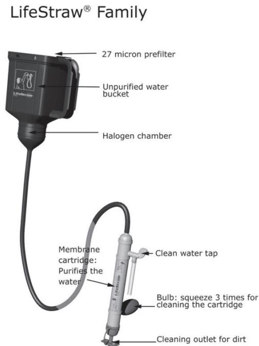
Figure 5: LifeStraw® schematic (Clasen et al., 2009, p. 820)
