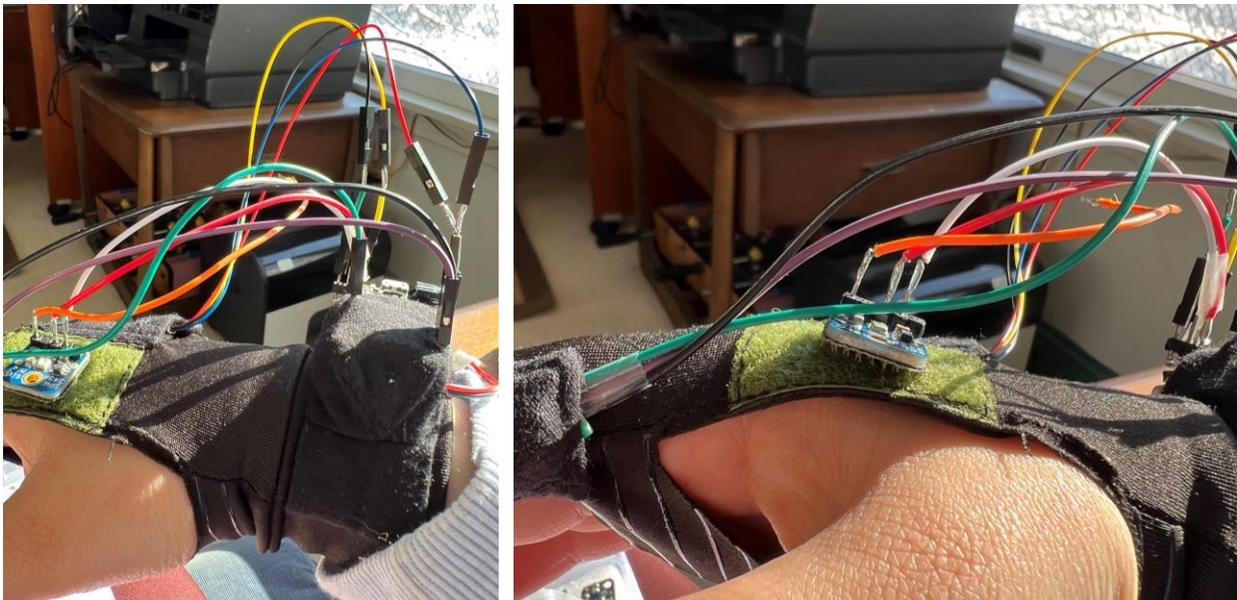
Additionally, these images show the high-winding nature of the wires; the system is not contained, and jumper wires with female heads have been used for trouble-shooting and testing.
