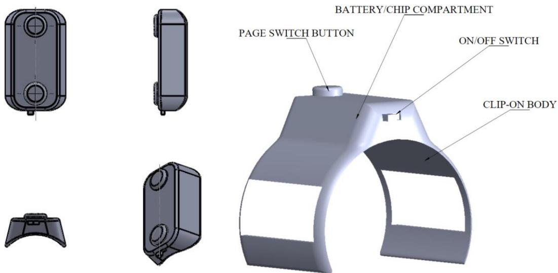
Fig. 1 First Designs of Instrument-Based Device
