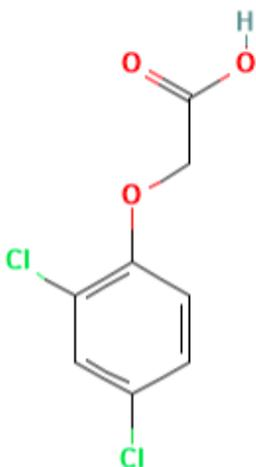
Figure 6. The chemical structure of 2,4-D. Image from PubChem and the National Center for Biotechnology Information (2022).
