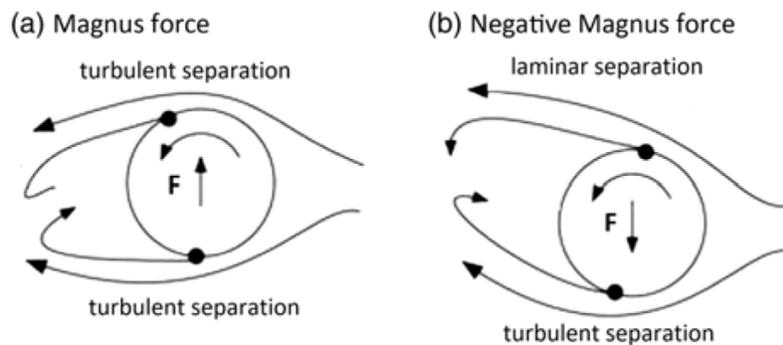
*Figure 6.* Magnus Force vs. Negative Magnus Force. From “Inverse Magnus effect on a rotating sphere: when and why,” by Kim, J., Choi, H., Park, H., and Yoo, J. Y., 2014, doi:10.1017/jfm.2014.428. Copyright 2014 by Cambridge University Press. Reprinted with Permission.
