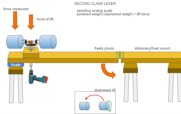
Figure 8. Magnus/Flettner Rotorcraft Testable Prototype. Own work.
