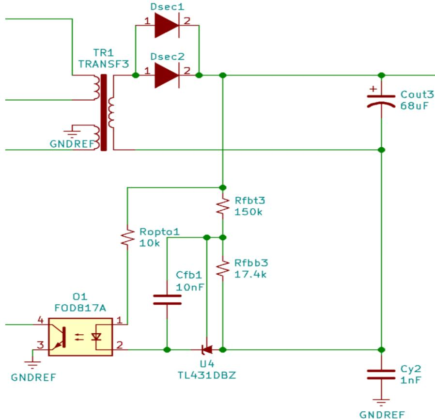
Fig. 7. Implementation of the output voltage feedback circuit.
