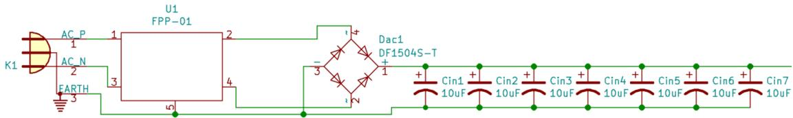
Fig. 5. Line filter and DC rectification implementation.
