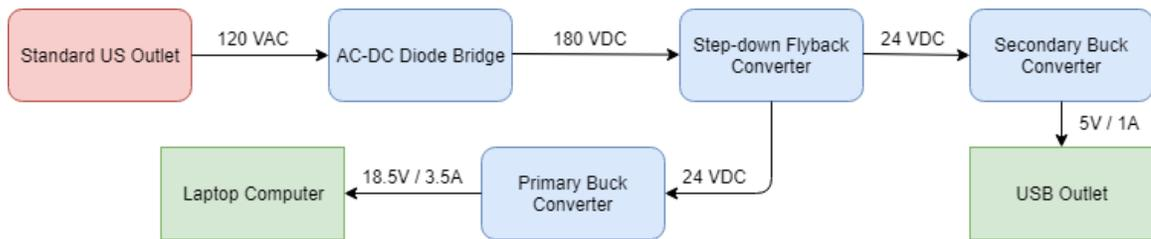
Fig. 1. The block diagram representing the converter architecture.
