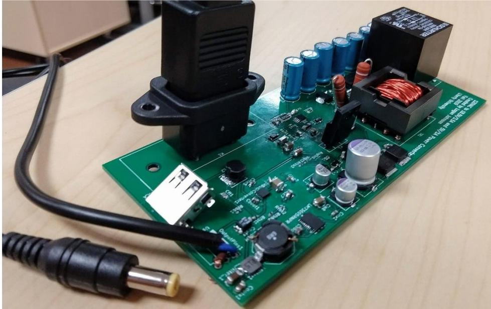
Fig. 10. The physical implementation of the power converter.
