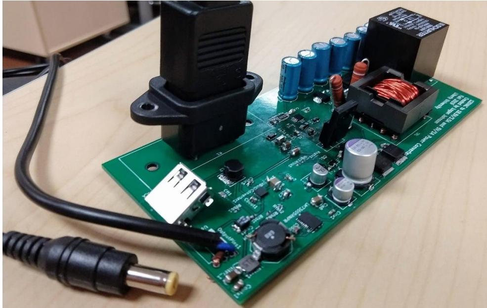
Fig. 10. The physical implementation of the power converter.
