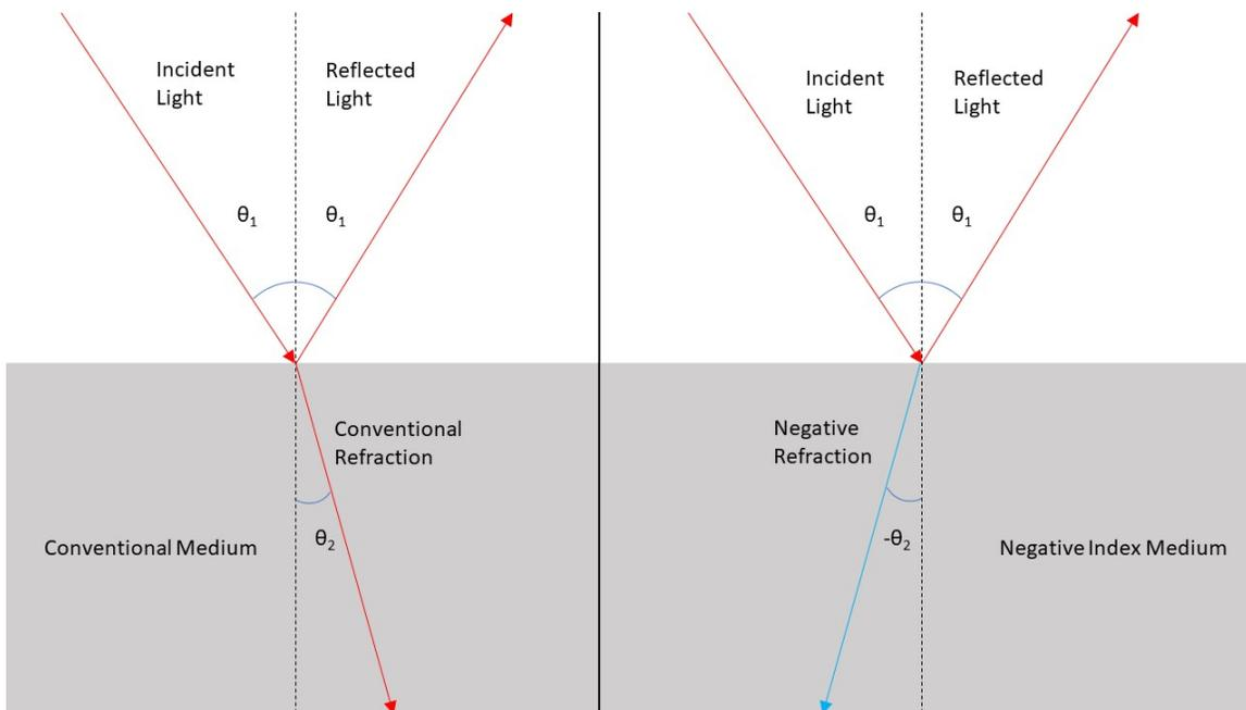
Figure 5: Refraction in conventional and negative index media.
