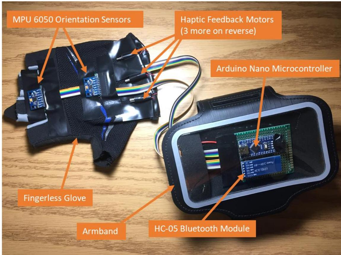
*Figure 1.* Visual prototype of design.
