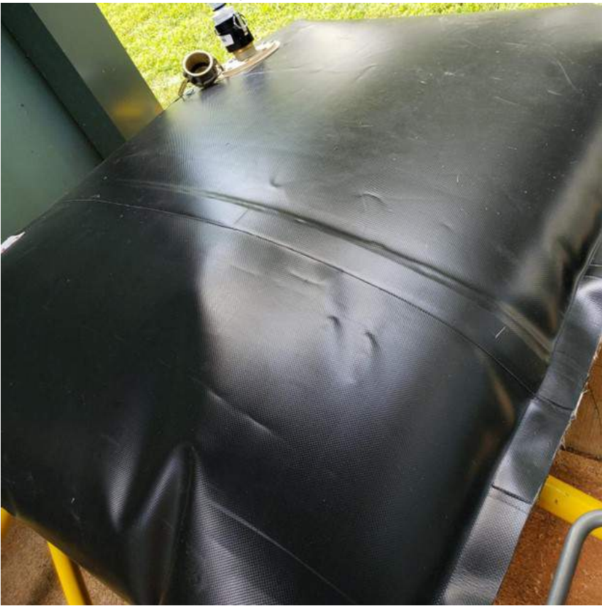
(B) Filled UDCN Bladder Tank
