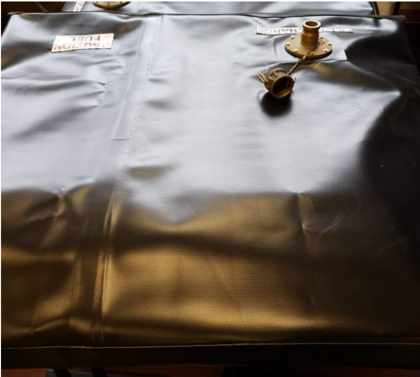
(A) 100-gallon UDCN Bladder Tank
