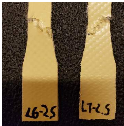
FIGURE 2.6: Longitudinal UDCN specimen fracture after 2.5 mm/min monotonic loading.
