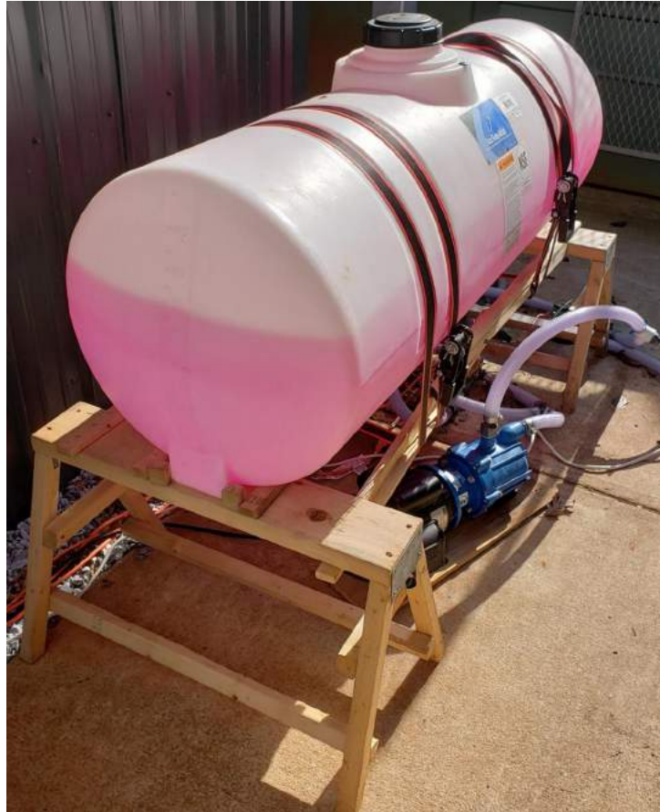
FIGURE 3.8: PPE Tank Filled with Antifreeze-Water Solution
