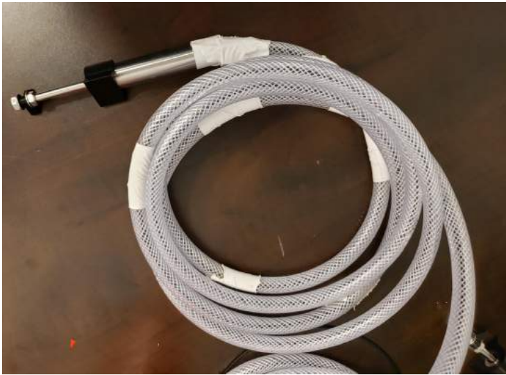
(B) LVDT Sensor Reinforced by Vinyl Tubing
