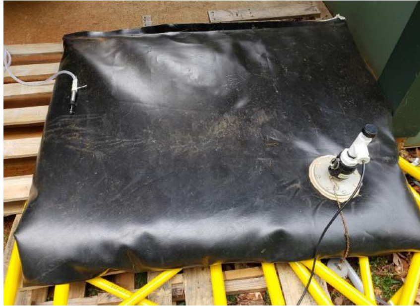
FIGURE 3.9: PSH loop testing with both tanks at ground level.
