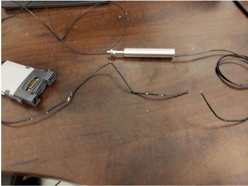
(A) LVDT Wiring Damaged by Squirrels
