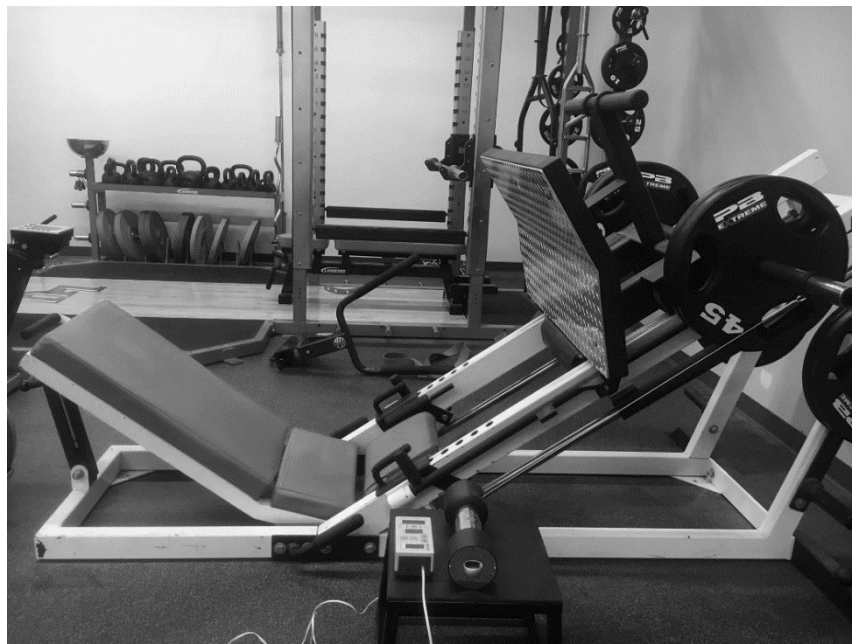
Figure 1. Nebula seated leg press machine with attached Tendo unit (Bouton, 2019).
