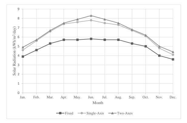
*Figure 4*. Monthly solar radiation received by Lynchburg collectors. The single-axis collectors offer significant improvement over fixed-axis collectors, but the two-axes collectors are only slightly better than the single-axis collectors. Data for figure retrieved from *Solar Radiation Data Manual for Flat-Plane and Concentrating Collectors* by Marion and Wilcox (1994), Golden, CO: National Renewable Energy Laboratory.
