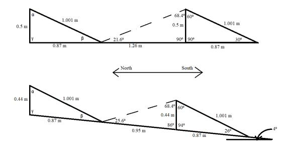
*Figure 5*. Solar collectors on a flat surface with a ground coverage ratio of 0.47 are above while solar collectors on a 4<sup>o</sup> slope are below. The collectors can be closer together on the sloped surface and still have the same amount of shade covering.
