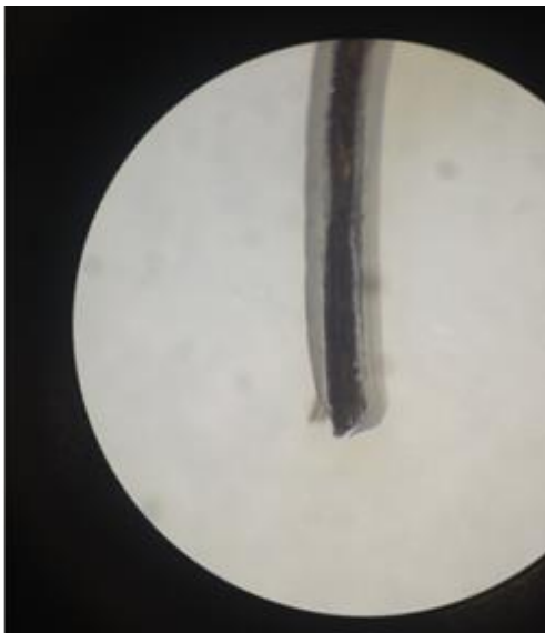
Figure 2. The tip of the piece of wire from a twist tie used in the experiment as seen under a dissecting microscope. The tip has a hook that is similar to the hooks on a tick's leg.
