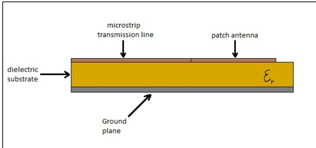
**Figure 7:** Typical Patch Antenna (Side View) (2014) Image adapted by the author from content at <http://www.antenna-theory.com/antennas/patches/antenna.php>
