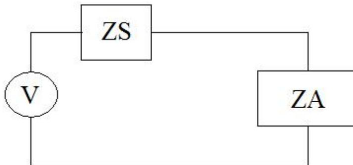
**Figure 3:** Impedance Model of an Antenna (2008)
