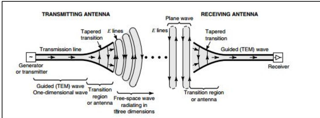
**Figure 2:** Transmitting and Receiving Antenna Model (2002)
