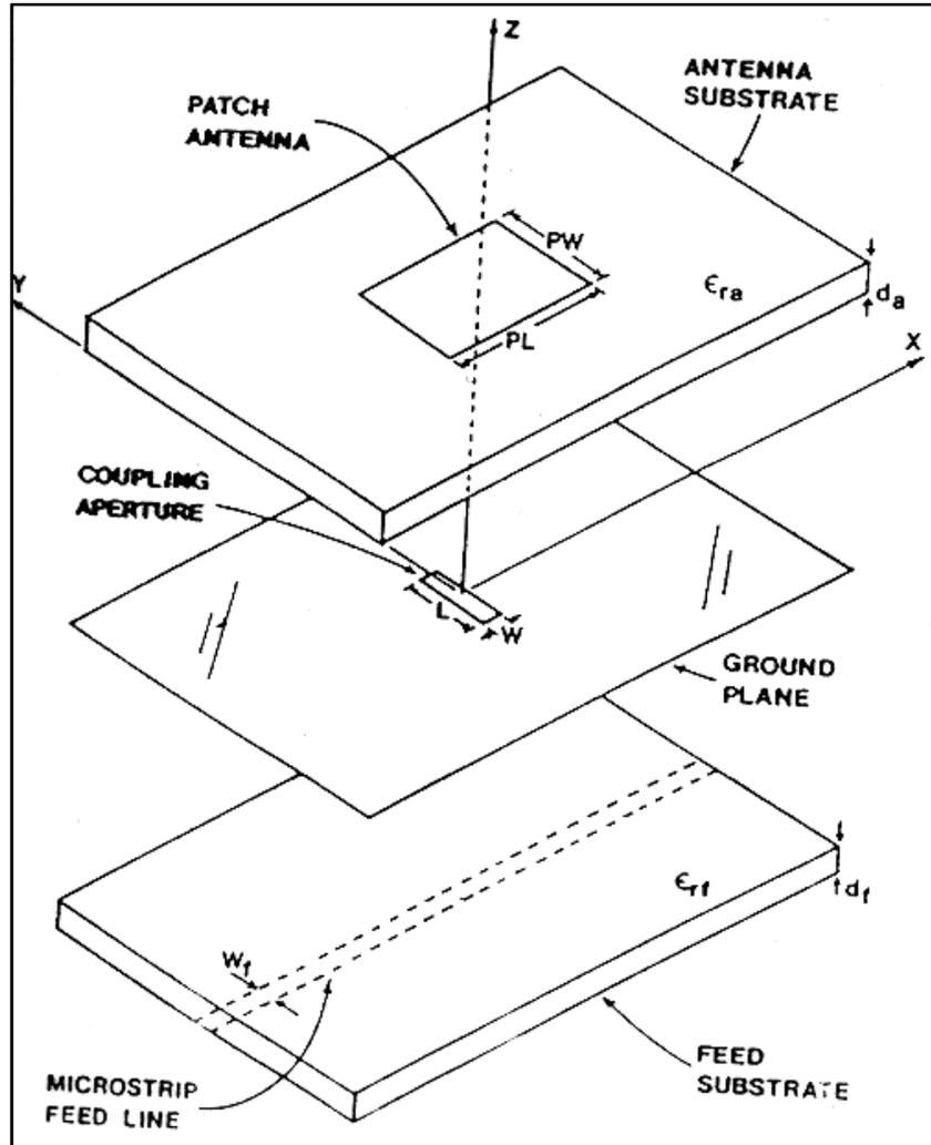
**Figure 8:** Alternative Patch Antenna Construction (Aperture-coupled) (n.d.)
