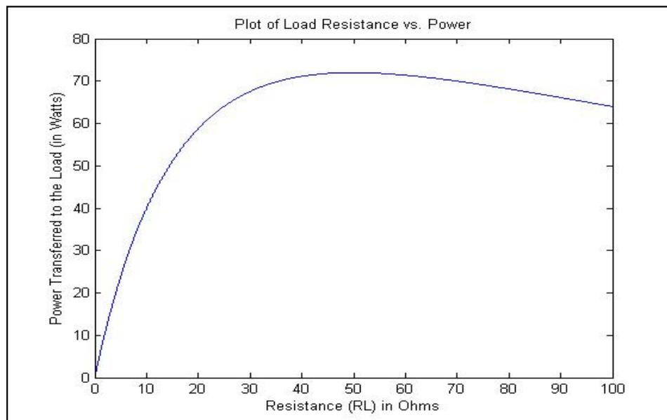
**Figure 4:** Plot of Load Resistance vs. Power (Graph Designed by the Author)
