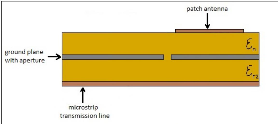
**Figure 11:** Aperture-fed Antenna Construction (Side View) (2014) Image adapted by the author from content at <http://www.antenna-theory.com/antennas/patches/antenna.php>
