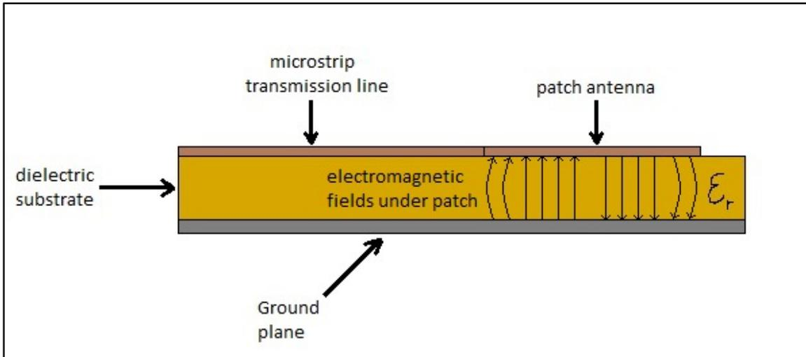
**Figure 9:** Fields inside a Patch Antenna (2014) Image adapted by the author from content at <http://www.antenna-theory.com/antennas/patches/antenna.php>
