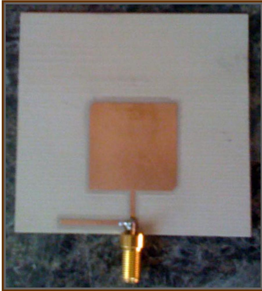
**Figure 6:** Patch Antenna Example (2008)
