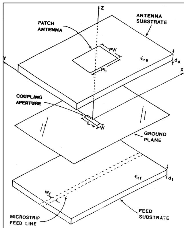
**Figure 10:** Alternative Patch Antenna Construction (Aperture-coupled) (n.d.)
