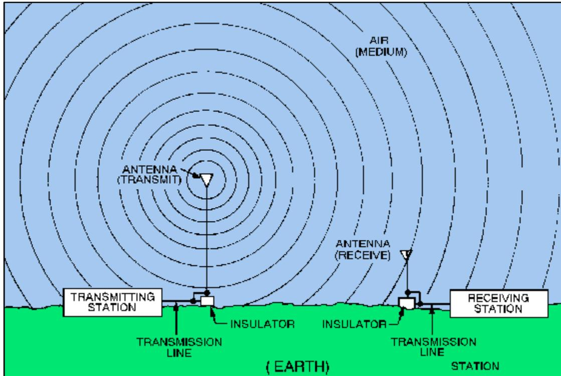
**Figure 1:** Transmitting and Receiving Radio Model (2011)
