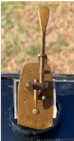
Figure 3. Author Alan Gillen's personal replica of Leeuwenhoek's microscope in Leiden. It has a 100x objective. Spirillum volutans can be seen with it.
