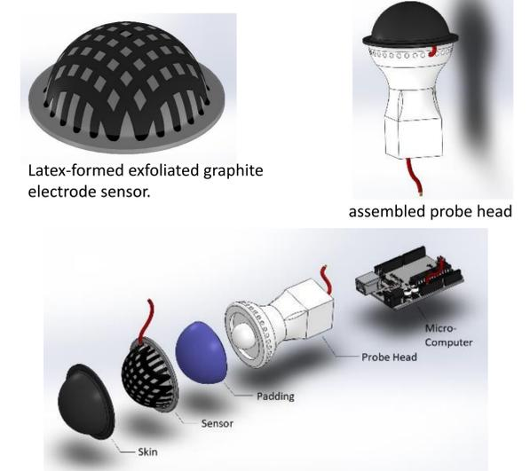
Figure 8. Schematic showing components of the palpable device
