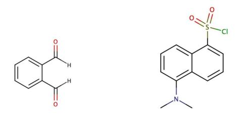
Figure 10. Derivatizing agents OPA (left) and dansyl chloride (right).
