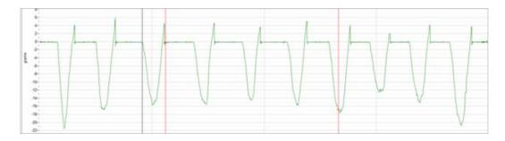
**Figure 3**. The results of the grams of force for the Window Fly Trap strips as recorded by the force transducer. The flat horizontal line is the baseline of zero, where no force was recorded. The negative spike is the force asserted as the wire was pressed onto the tape, and the positive spike is the amount of force needed to pull the wire off of the tape. This peak is a measure of how sticky the tape is. This explanation of the graph is applicable to each of the following figures.
