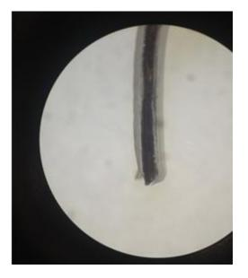
**Figure 2.** The tip of the piece of wire from a twist tie used in the experiment as seen under a dissecting microscope. The tip has a hook that is similar to the hooks on a tick's leg.
