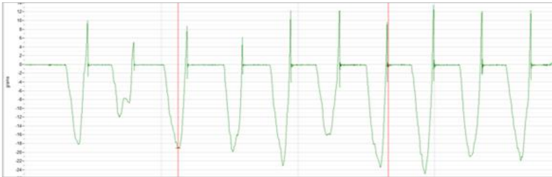
Figure 5. The results of the grams of force for the yellow lab tape as recorded by the force transducer.
