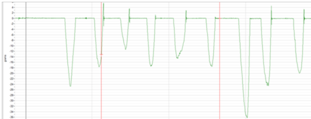
Figure 7. The results of the grams of force for the clear packing tape as recorded by the force transducer.
